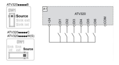
Switch SW1 set to "Source" position and use of an external power supply for the DIs.
