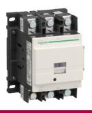
Contactor, TeSys Deca, 3P(3NO), AC-3, <=440V, 115A, 125V DC standard coil, lugs/bars terminals, without front cover
