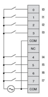
The two COM terminals are not connected together internally.
