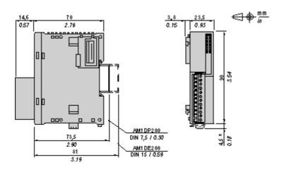
NOTE: \* 8.5 mm (0.33 in) when the clamp is pulled out.
