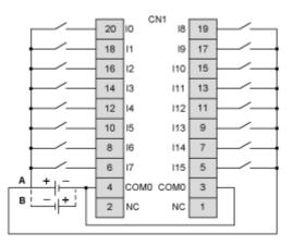
The COM0 terminals are connected internally
